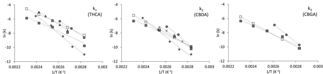
**Figure 5.** Arrhenius plots for THCA (left), CBDA (middle), and CBGA (right). (■) This work (simple model); (□) this work (mass balance model); (●) Wang et al.;<sup>17</sup> (◆) Veress et al.;<sup>14</sup> (▲) Perrotin-Brunel et al.;<sup>15</sup> (\*) Citti et al.<sup>16</sup>
