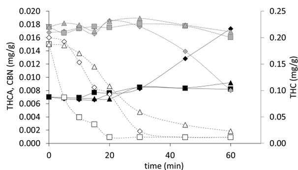
**Figure 2.** THC (gray), THCA (empty) and CBN (black) concentrations during decarboxylation at 140 °C: (◆) open beaker, thin bed; (▲) open beaker, deep bed; (■) N<sub>2</sub>-sealed pouch.
